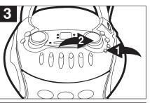
Press the REPEAT button ① once, the REPEAT indicator will blink and the unit will play the selected track over and over until the STOP (■) button ② is pressed.
